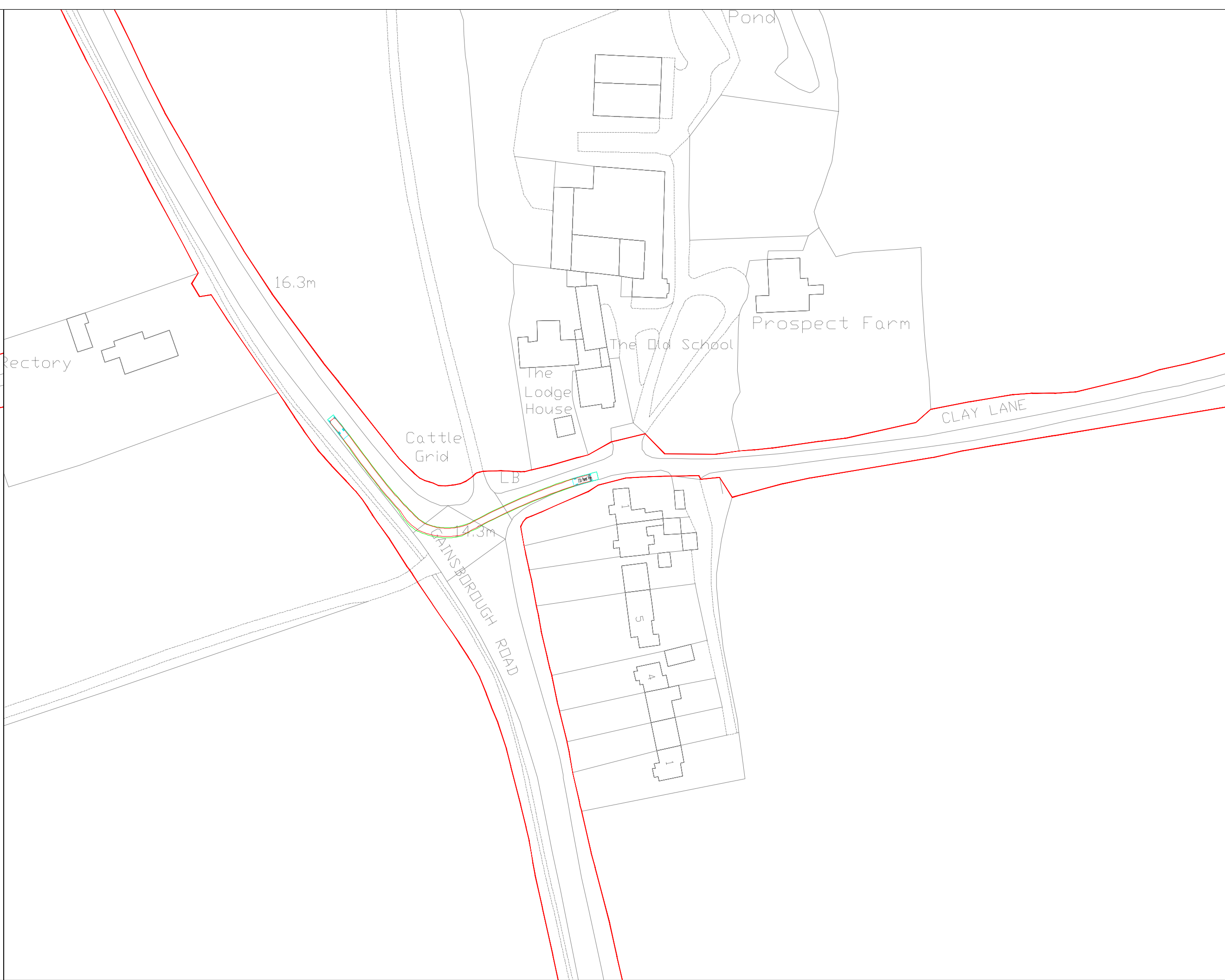
7.5t PANEL VAN VEHICLE MANOUVRE, HEADING WEST OUT OF CLAY LANE TURNING RIGHT ONTO ON GAINSBOROUGH ROAD A156 HEADING NORTH - SCALE 1:1000
